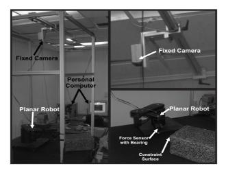
Fig. 2. Experimental setup
