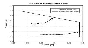
Fig. 7. Cartesian robot task in robot space (m).
