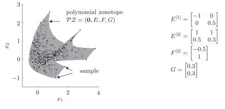
Figure 7: Over-approximative plot of a polynomial zonotope as specified in the figure. Random samples of possible values demonstrate the accuracy of the over-approximative plot.
