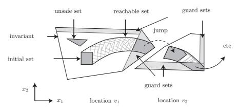
Figure 18: Illustration of the reachable set of a hybrid automaton.
