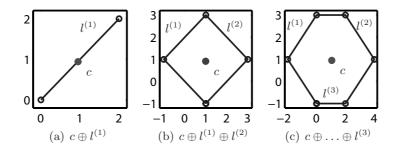
Figure 3: Step-by-step construction of a zonotope.
