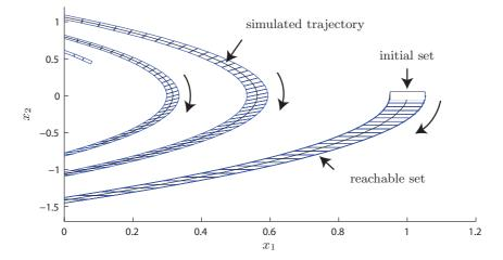
Figure 20: Illustration of the reachable set of the bouncing ball. The black box shows the initial set and the black line shows the simulated trajectory.
