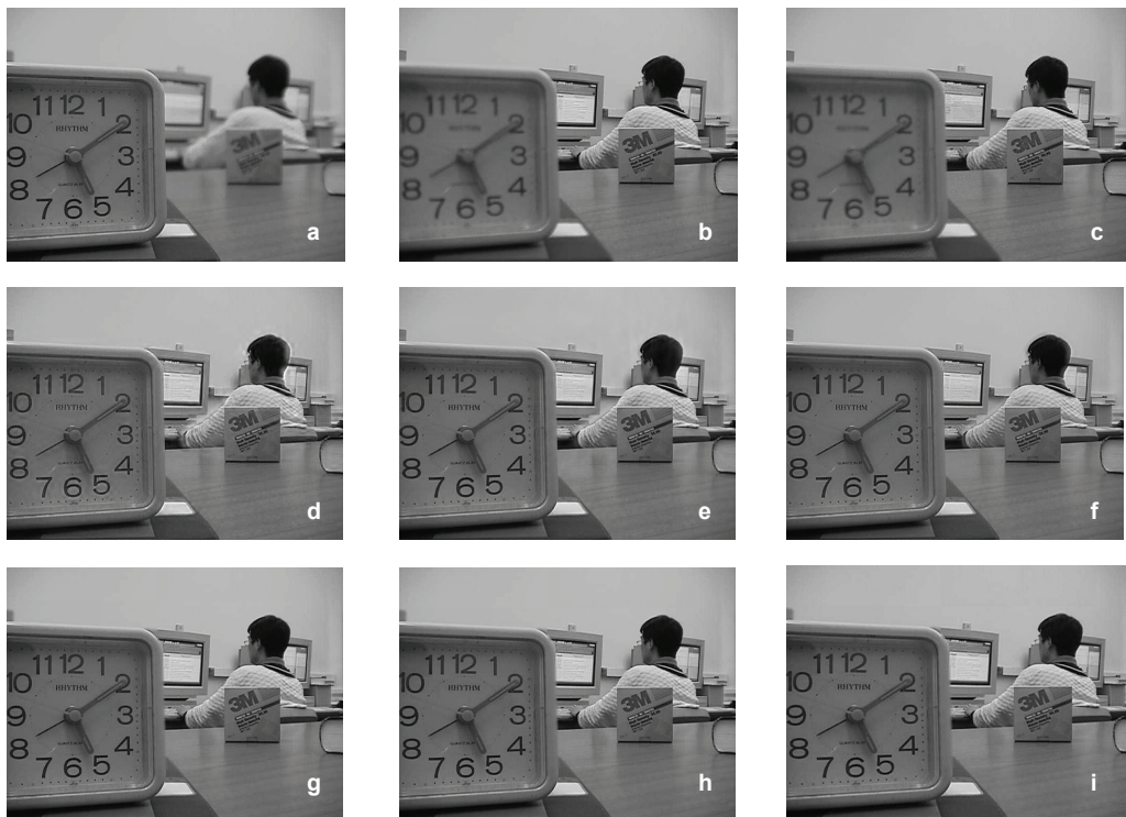
Fig. 5. Digital camera image fusion. Source image (focus on the clock, size of 480 \times 640 ) – a; source image (focus on the student) – b; auto-focus image – c; fused image obtained by DWT algorithm – d; fused image obtained by CT algorithm – e; fused image obtained by NSCT algorithm – f; fused image obtained by NSCT-PCNN algorithm – g; fused image obtained by GA algorithm – h; fused image obtained by BPSO algorithm – i.
