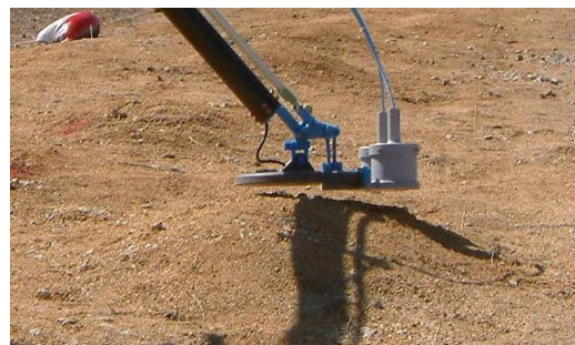
Fig. 9. The sensor head closely follows the contour of the terrain.
