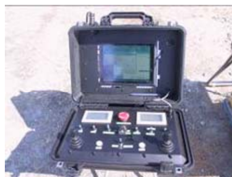
Fig. 4. The remote controller is equipped with two joysticks and few switches. The display panel is in fact a panel computer
