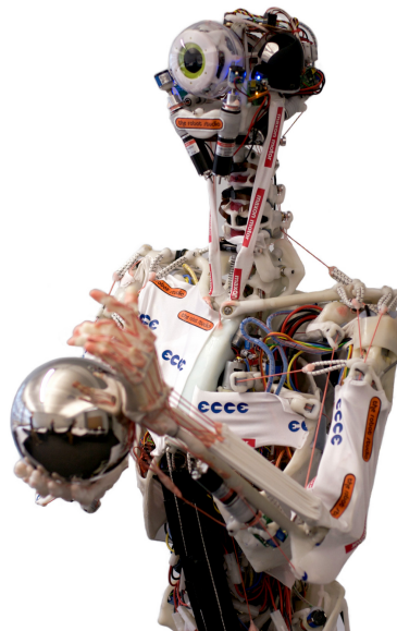
Fig. 1. ECCEROBOT Design Study (EDS). This is the newest platform in the ECCEROBOT family [3]. In this type of robot not only the appearance of the human body is mimicked but also the inner structures, like bones, joints, muscles, and tendons.
