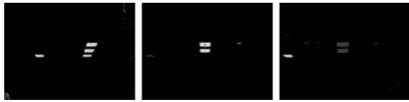
Figure 9. Similarity of pixels to the colors “blue”, “yellow”, and “red” (from left to right) of the image in Figure 7. The colors “yellow” and “red” are similar enough to still yield a low ranking for their counterparts.
