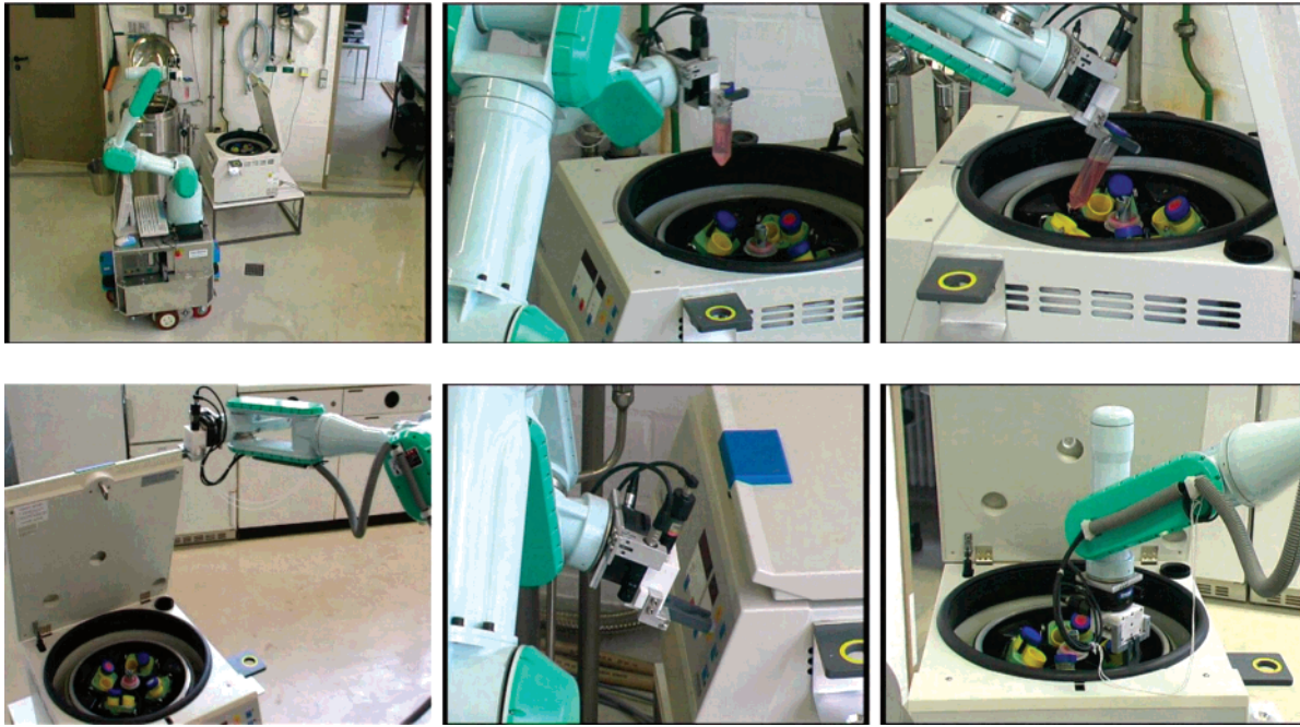
Figure 18. Operating the centrifuge. Image sequence (from left to right and from top to bottom) showing the robot (i) approaching the centrifuge and determining its position and orientation, (ii) analyzing visually the orientation of the turntable in the centrifuge, (iii) putting the vial into one of the vial holders of the centrifuge, (iv) closing the cover of the centrifuge without any further help or tool, (v) pushing the buttons of the centrifuge to start its operation, and (vi) slightly rotating the turntable of the centrifuge to enable a safe retraction of the vial after having stopped the centrifuge and let it come to a standstill.
