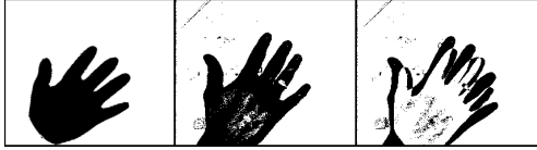
Figure 2: Example of pixel-level measurement. Left: expected object shadow, Middle: foreground segmentation on the real image; Right: residual image.
