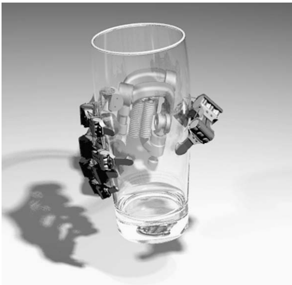
Fig. 11. Final hand design virtually grasping a 0.51 glass.
