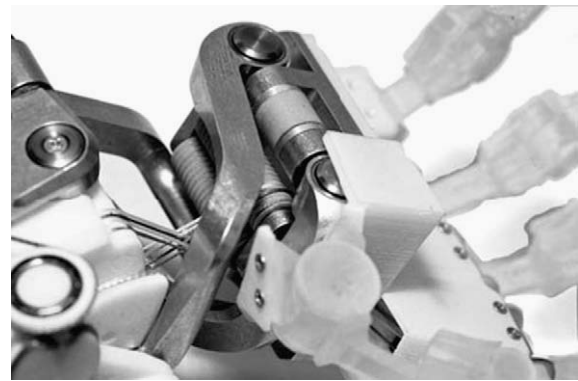
Fig. 12. Wrist integrated in forearm mockup.
