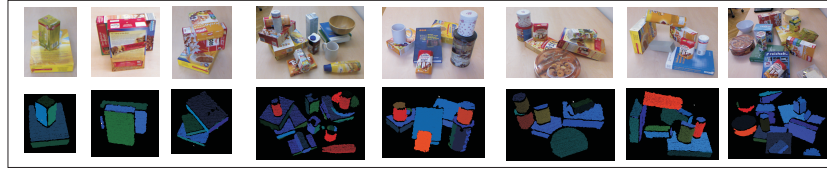
Fig. 6. Primitive Shape Detection results. Cylinders are shown in red and planes are shown in blue-green.
