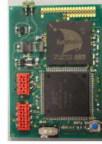
smallest (1 chip, 18 core) and largest (48 chip, 864 core) Spinnaker board
